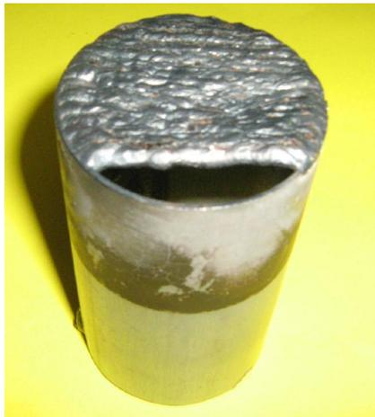
Top Left picture: Shows the inside of the exhaust pipe after it has been welded over, No burn through NO bubbles only slight discoloration.
