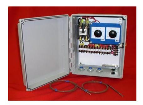
The fiberglass enclosure is UL/CSA listed for use in NEMA 4, 4X, 12 and 13 environments. Employing two electronic controllers, the assembly can be used for a variety of tank and pipe heating applications requiring reliable control. Components carry UL, CSA, and CE approval with internal wiring that is NEC and IEEE compliant. The complete assembly can be provided with a UL/CUL approval stamp per customer request.
